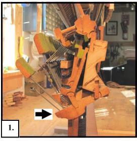
If the action of an upright piano is removed for servicing and a bridle strap is broken or missing, the lower portion of the mechanism (the wippen) will swing down.
