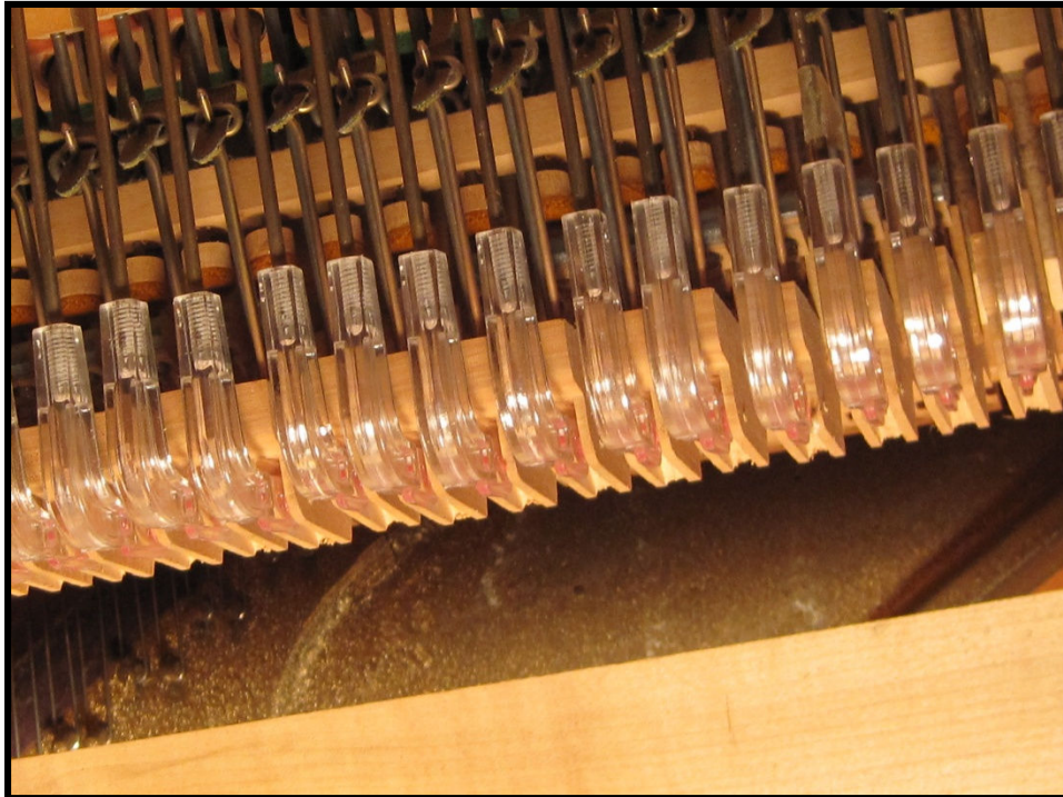
A completed installation of Vagias Snap-On elbows in a spinet piano.
