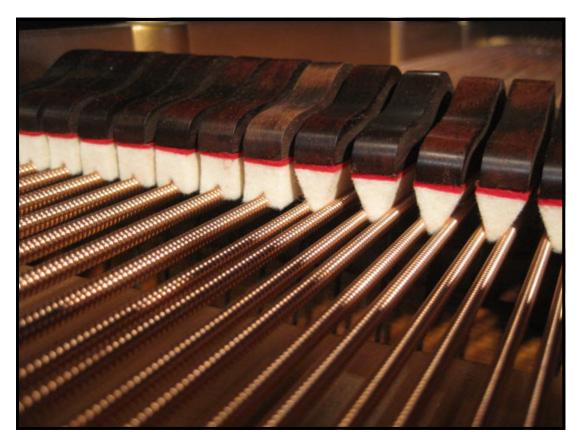
A new set of dampers installed and ready quiet things down when needed.
